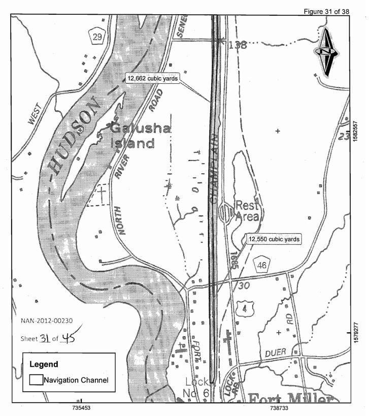
All bathymetry excluding the Fort Edward Yacht Basin is based on a 2009 survey performed by the NYSCC. The Fort Edward Yacht Basin survey was performed in 2010 and 2011. Volumes provided are calculated with the navigational design depth of the Champlain Canal of 12 feet plus a 2 foot overcut, for a total depth of 14 feet.
