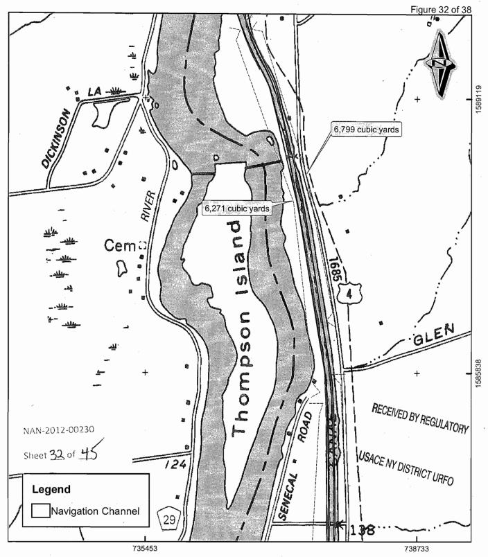
All bathymetry excluding the Fort Edward Yacht Basin is based on a 2009 survey performed by the NYSCC. The Fort Edward Yacht Basin survey was performed in 2010 and 2011. Volumes provided are calculated with the navigational design depth of the Champlain Canal of 12 feet plus a 2 foot overcut, for a total depth of 14 feet.
