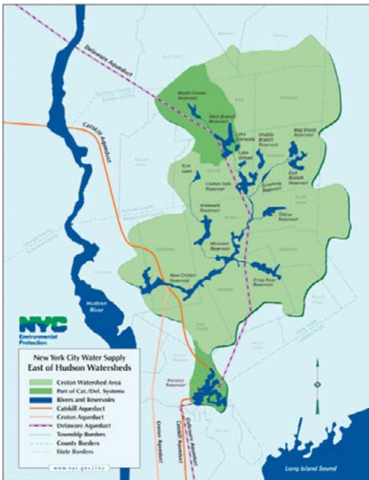
Figure 2: Map of Croton Watershed East of the Hudson River, the 375-square-mile Croton Watershed typically supplies 10% of the City's daily water supply from sources in Westchester, Putnam and Dutchess Counties. The Croton system remains unfiltered and offline as of the release of this report, although a filtration plant for that system is currently under construction and scheduled to go on-line in August 2013.
